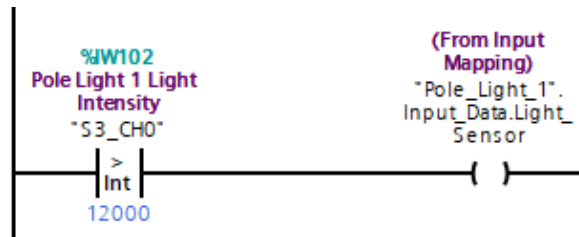
Figure 2.5 – Analog alternative – when above 12mA, consider the light sensor as active and write it to the appropriate variable in the dataset
